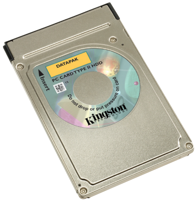
FIG. 1. The Kingston DataPak 5GB Type II PC Card uses a 1.8” Winchester hard drive spinning at 3,990 rpm. It has a mean time between failure (MTBF) of over 300,000 hours and a data reliability of 1 non-recoverable error in 1013 bits read. (Photo courtesy of Kingston Technology Company, Inc.)
