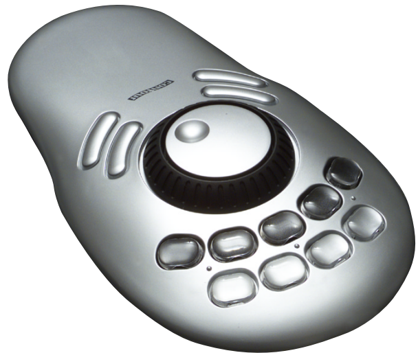
FIG. 1. The central control element of the Contour ShuttlePRO is the jog wheel and shuttle knob. The shuttle knob is the outer ring that controls the rapid forward or rewind of digital frames. The jog wheel, located in the center of the knob, provides precise frame-by-frame control. (Photo courtesy of Contour Design Inc.)
