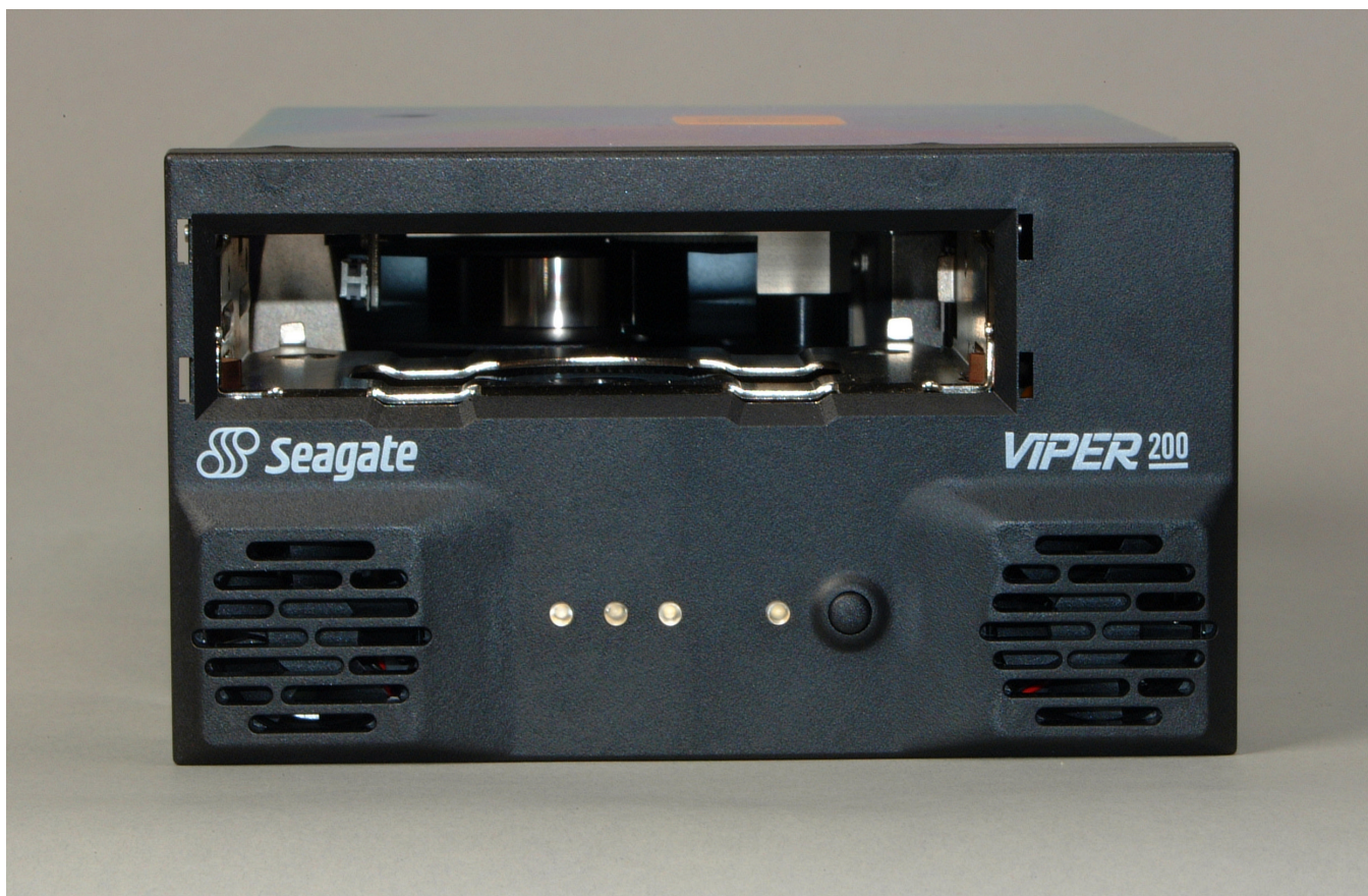
FIG. 5: Front view of a Seagate Viper LTO tape drive. (Photo courtesy of Fuji Photo Film U.S.A., Inc.)
