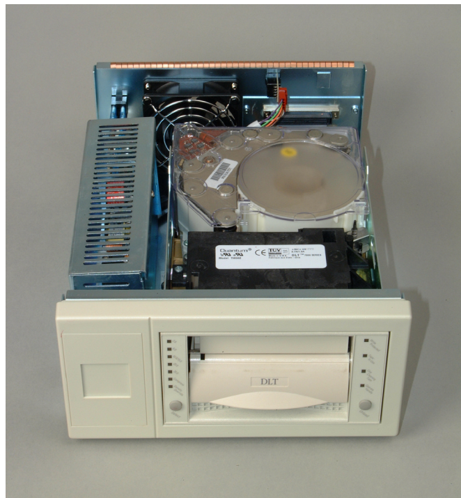
FIG. 3: Front view of a Quantum DLTape 7000 drive without the external cover. (Photo courtesy of Fuji Photo Film U.S.A., Inc.)
